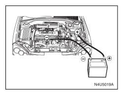
6) Connect the red positive (+) cable to the positive (+) terminal of the dead battery. Use a remote positive (+) terminal if the vehicle has one.
